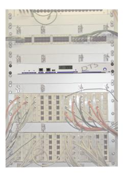
DTS device mounted in a 19" IT-Rack
